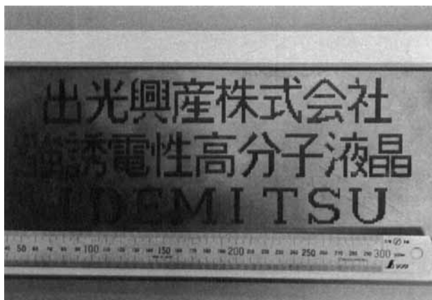
Figure 11. Photograph of a dynamically driven, simple, matrix display (15 cm \times 40 cm, 100 \times 300 pixels).
